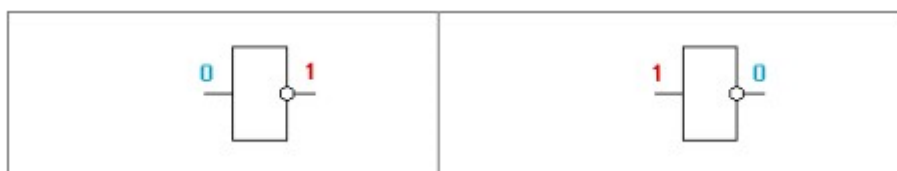
5.74-rasm. Inverterni ishlash prinsipi
