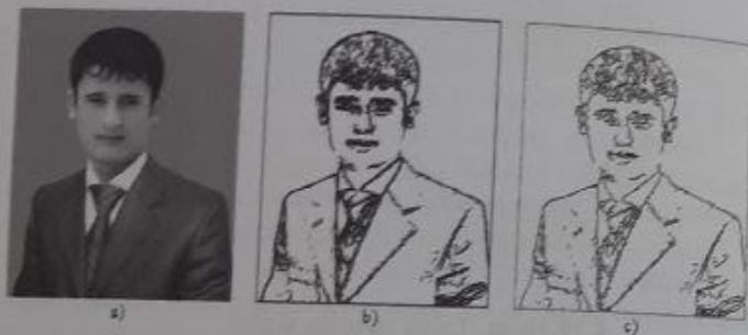
4.30-rasm. Berilgan tasvir (a), uning konturi natijasi (b) hamda uning ingichkalashtirilgan (skelet) natijasi (c).
