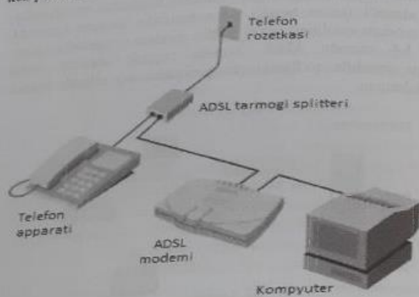
5.5-rasm. Abonent inshootida ADSL modem va uning komponentalarini ulanish ketma-ketligi
