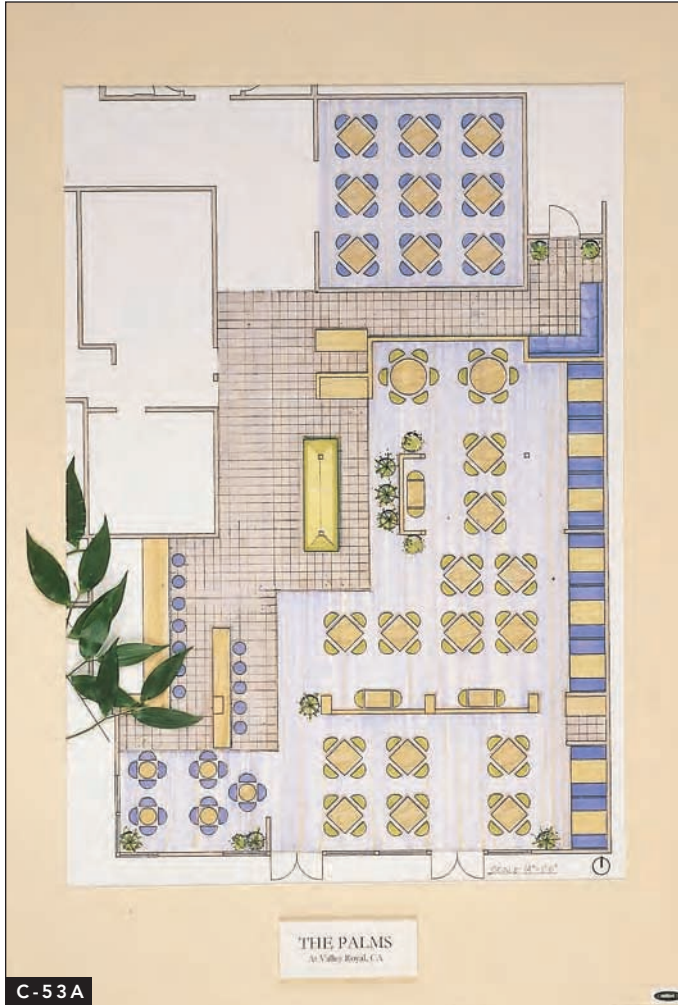
FIGURES C-53A, C-53B Final presentation boards for a hospitality project containing drawings that are window matted and samples that are surface mounted, including actual plant materials. Drawings for this presentation were mounted not with spray adhesive but with limited amounts of double-sided tape to prevent warping.
