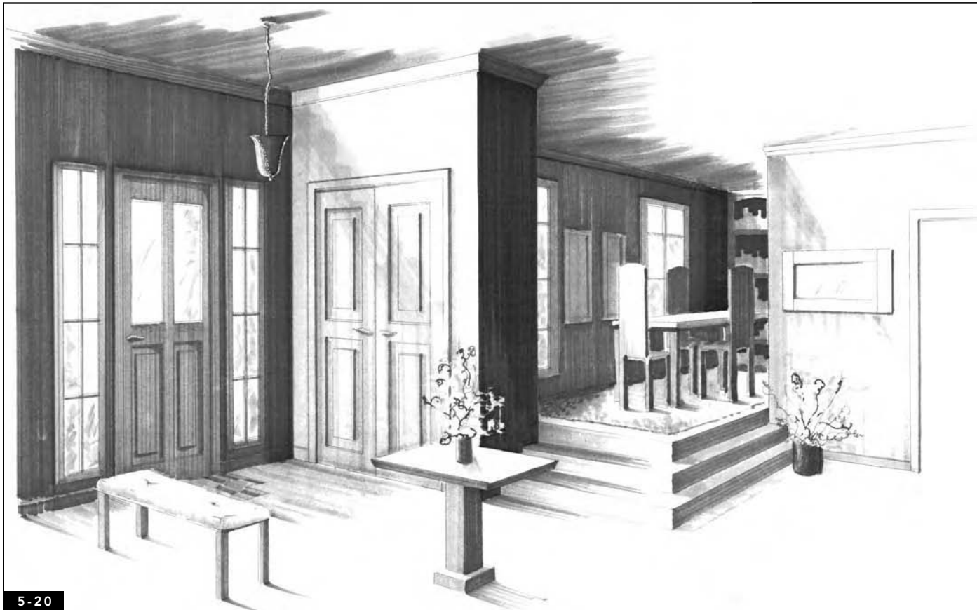
FIGURE 5-20 This gray marker rendering was created using gray markers and a small amount of white pen (for the light fixture) on marker paper. Drawing and design by Kristy Bokelman.
