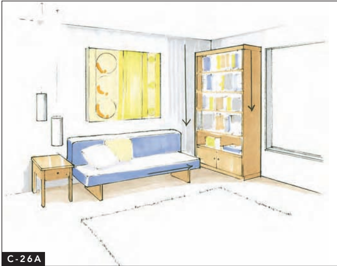
FIGURE C-26A The first steps in rendering this two-point perspective on bond paper involved laying in general background material hues in values lighter than the final will depict. A straightedge was used for marker application in the directions shown. The top surfaces of the sofa and floor were left blank to prepare for the use of dry (chalk) pastels. Simple shadows were laid in with warm gray marker on the floor, while the wall surfaces received cool gray markers.
