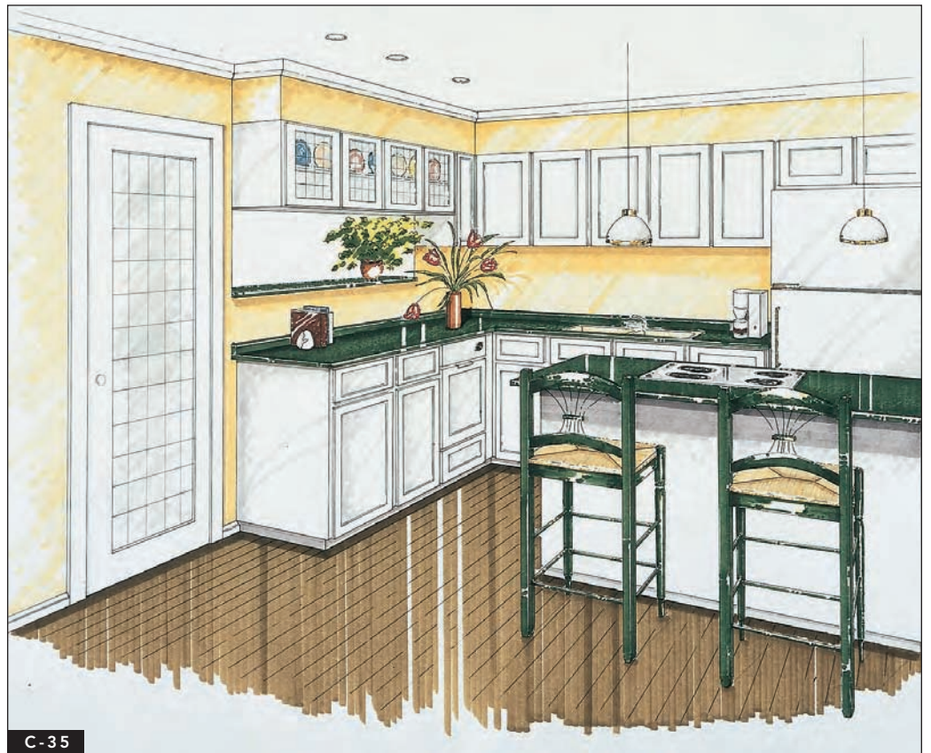
FIGURE C-35 Rendered perspective included in student design-development presentation. Marker and pencil on bond paper. Notice the vertical application of marker and portions of paper left blank to serve as highlights. Design and rendering by Susan Reische.
