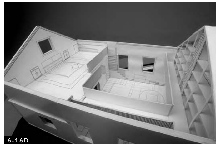
FIGURES 6-16A, B, C, AND D This foam board and paper model was built to depict the design of a small two-story building. Due to the nature of the design and the scale of the project, the model was designed in two parts, the top of which can be removed for better viewing of the first story. Special care was given to accurately portray specially designed cabinetry and millwork details. Design and model by Siv Jane Refsnes. Photograph by Bill Wikrent.
