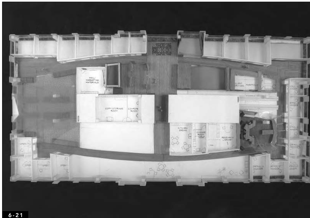
FIGURE 6-21 An overhead view of a large study model built for a professional project, constructed of bond paper, foam board, plastic, teak veneer, metal screen, and fabric. Design and model by Meyer, Scherer, & Rockcastle, Ltd. Photograph by Bill Wikrent.
