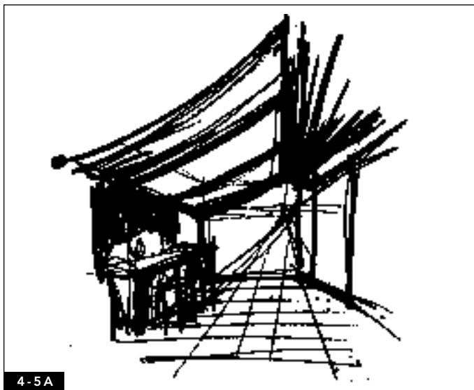
FIGURES 4-5A, 4-5B Practicing estimated one-point sketching leads to the ability to do quick sketches in client and team meetings. This group of drawings was sketched in less than ten minutes using ink pens.
