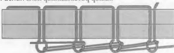
16-rasm. Ikki ipli zanjirsimon baxyaqator.
