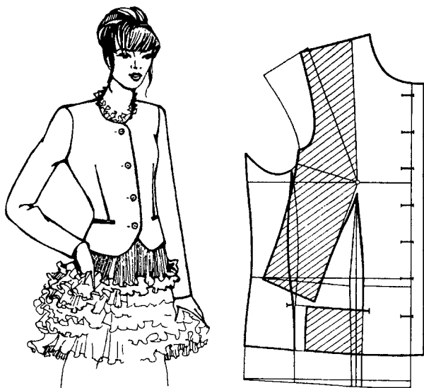
3.4-rasm. Cho'ntak chizig'iga o'tadigan bel vitachkasiga ko'krak vitachkasini o'tkazish.
