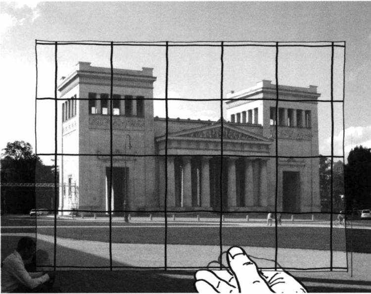
Fig. 81: Using a sheet of film with a grid of lines that divides up the building, which is distorted in perspective, into areas of equal size
