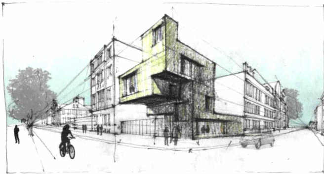
Fig. 89: Photograph of the empty site, construction of the perspective, insertion of the design volume, developing the image, completing the illustration
