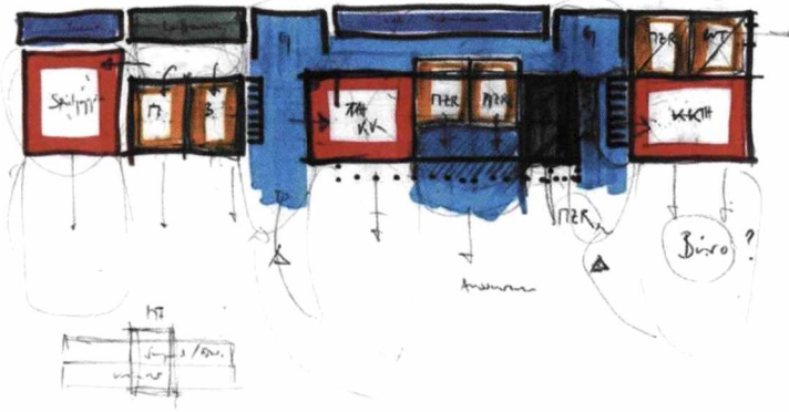
Fig. 48: A floor plan takes shape through the arrangement of rooms, sorted by colour according to their function.
