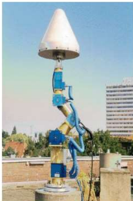
13.17-rasm. Haqiqiy vaqtda antennani absolyut sozlash uchun qurilma ( http://www.geopp.com/gnpcvdb/AOA_DM_T/ )
