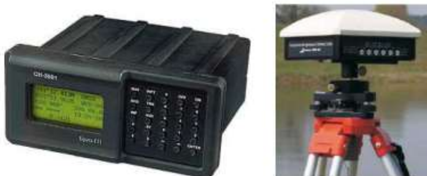
13.16-rasm. CH-3601 KB (" NAVIS ") chapda va GEO-161 OAJ "RIRV" Rossiya geodezik priyomniklari
