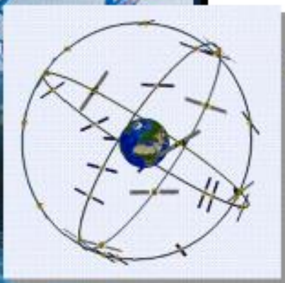
GPS Nominal Constellation 24 Satellites in 6 Orbital Planes 4 Satellites in each Plane 20,200 km Altitudes, 55 Degree Inclination
