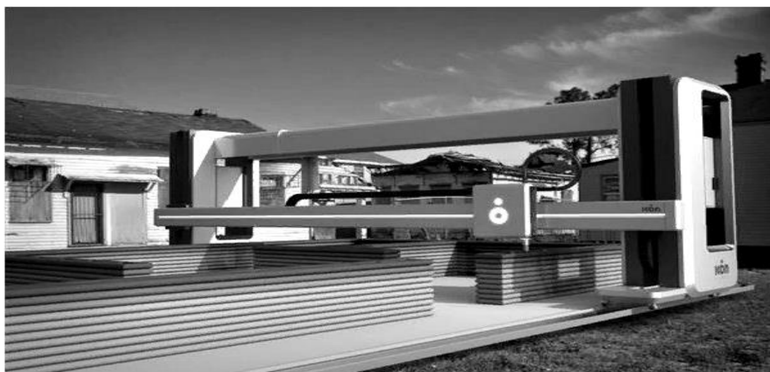
1.1.2.-rasm. 3D - qurilish materiallari ishlab chiqarish uchun printer Manba: hi-news.ru
